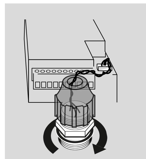
For the round call button, make sure that the sealing rubber is seated between the front panel and the nut.
