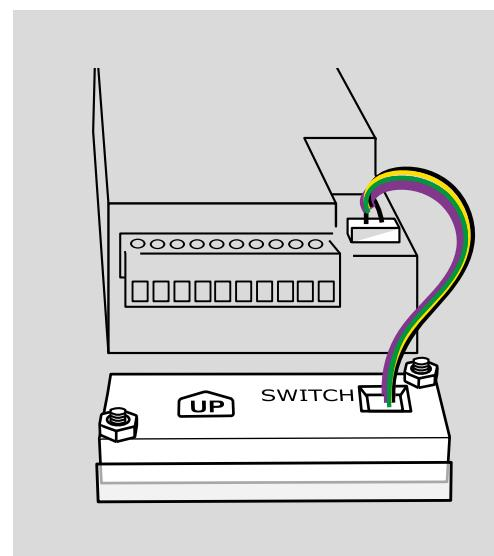
Use the four-wire cable from the "CB" port of the door station to connect a single call button.
