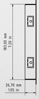
General tolerance DIN/EN 2768 -mK Wall cut-out dimension +4 mm/0.15 in Important note for cavity mounting (e.g. in pedestals and mailboxes):
