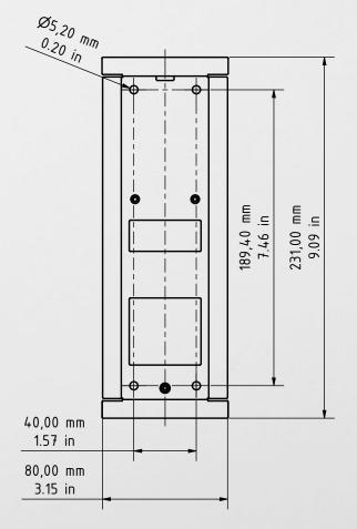
General tolerance DIN/EN 2768 -mK Wall cut-out dimension +4 mm/0.15 in
