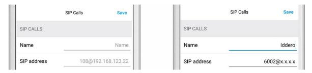
5. In the subsequent screen, enter an arbitrary name in the "Name" field, e.g. "Iddero". For the SIP address, enter the IP address or URL of your SIP server provider, prefixed with the SIP user id of your Iddero TouchOne panel and an "@"-symbol, e.g. "6002@x.x.x.x".
