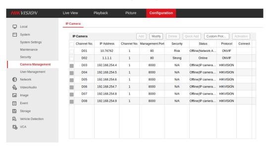
6. Here, set the "IP Camera-Address" to the IP address of your DoorBird IP Video Door Station and make sure "Protocol" is set to "ONVIF". Change the "User Name" to the App user from the "DIGITAL PASSPORT" document that was shipped with your DoorBird IP Video Door Station, e.g. "user0001". Enter the password associated with the App user into the "Password" field and confirm it in the field below. Close the window by clicking "OK".
