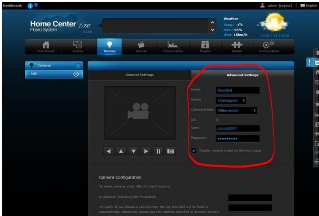
5. Scroll down to the “Camera Configuration” area and enter the IP address of your DoorBird IP Video Door Station into the “IP Address” field.
