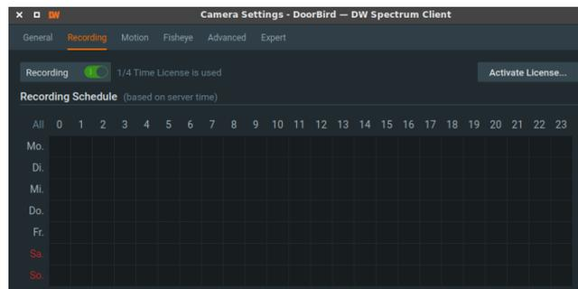
7. If your DoorBird IP Video Door Station supports continuous recording, edit the schedule settings to your preference. If your DoorBird IP Video Door Station does not support continuous recording, or if you prefer using event-based recording, proceed to step 3.1.
