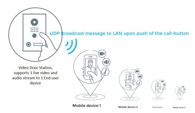
The mobile devices (e.g. smartphone, tablet, smart-home panel) listen for UDP Broadcast messages within the LAN from the door station. If a valid UDP Broadcast message (valid: fits to the call-button number) is received from the door station by the mobile devices, then the mobile devices play a "ding-dong" notification sound and offer the End-user the possibility to take the call upon user-interaction by e.g. pressing a button on the mobile devices.
